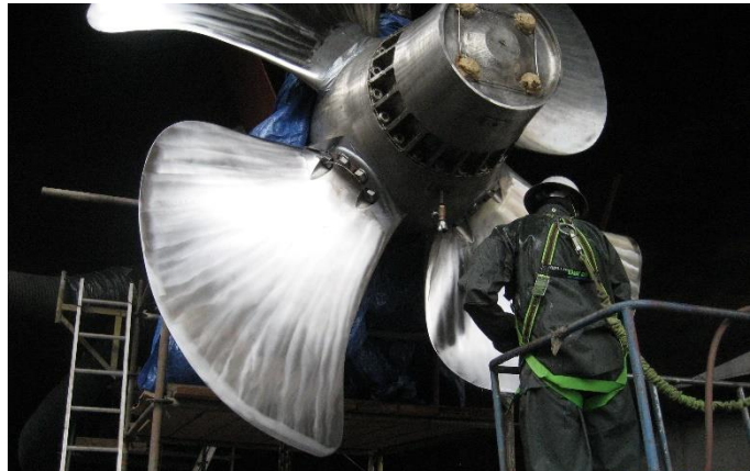
A shipyard worker polishing the wheels on the M/V Columbia while in drydock.
