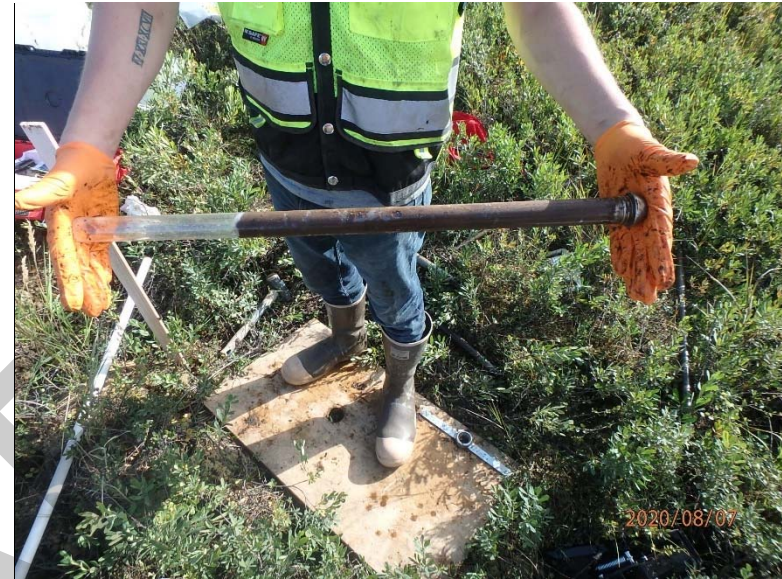
Typical sampling recovery using the drive hammer and PFAS-free liners
