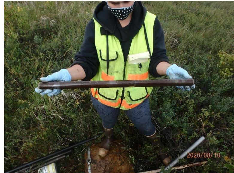
PFAS-free liner with highly compacted peat. Notice the slight bulge
