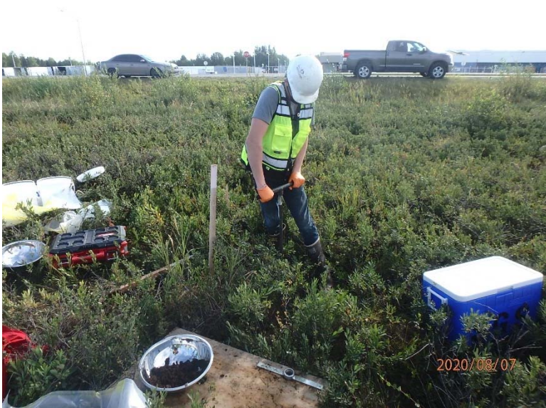
A bucket auger was used at this location because of too compaction issues using the drive sampler
