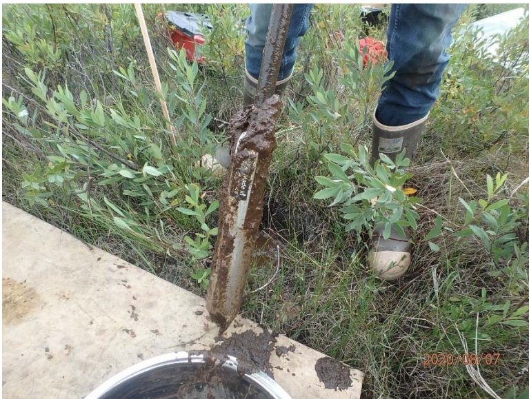
Depending upon material wetness, RSE sometimes sampled using a bucket auger
