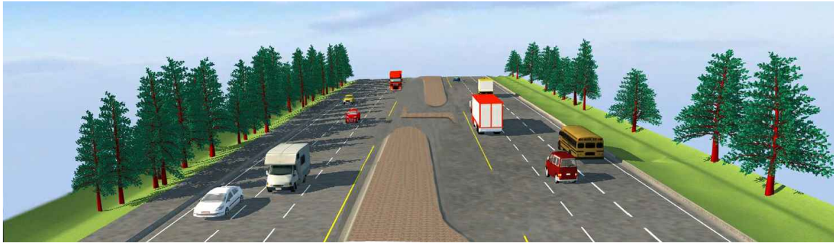
6-LANE URBAN SECTION RAISED MEDIAN WITH MULTI-USE PATHWAY BEHIND CURB (FULL BUILD-OUT)
