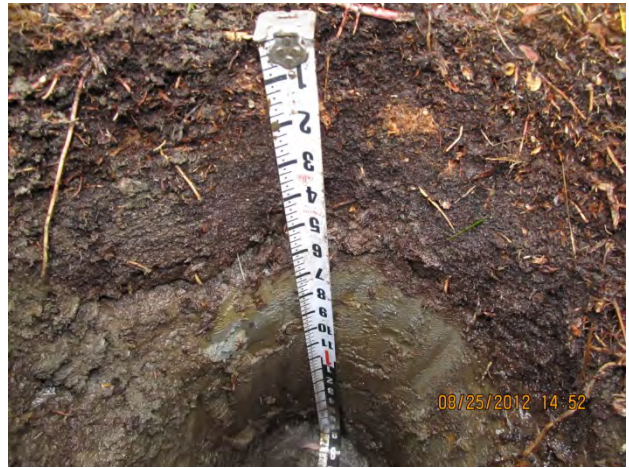
Hydrology: Saturated (A3) with shallow aquitard (D3) Soils: Organics over silty clay loam (Alaska Gleyed A13)
