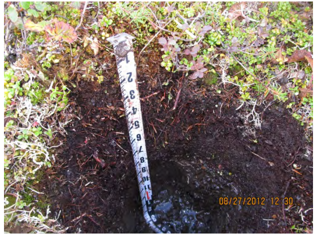
Hydrology: Saturation (A3) with shallow aquitard (D3) Soils: Organics over silty clay loam (Histic Epipedon A2)
