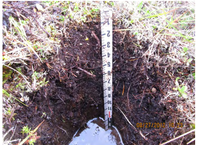
Hydrology: Saturation (A3) with a high water table (A2) Soils: Organics over silty clay loam (Histic Epipedon A2)
