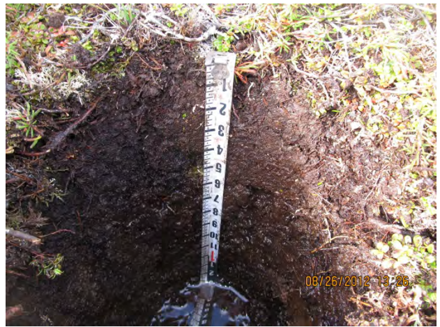
Hydrology: Saturated (A3) with high water table (A2) Soils: Organics over silty clay loam (Histic Epipedon A2)
