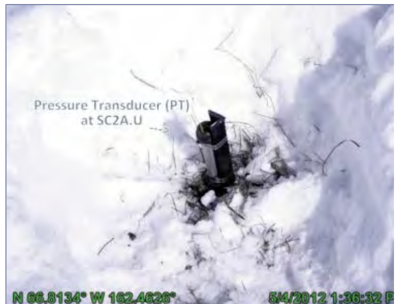
PHOTO 3.2: PT ASSEMBLY INSTALLED AT SC2A.U; MAY 4, 2012
