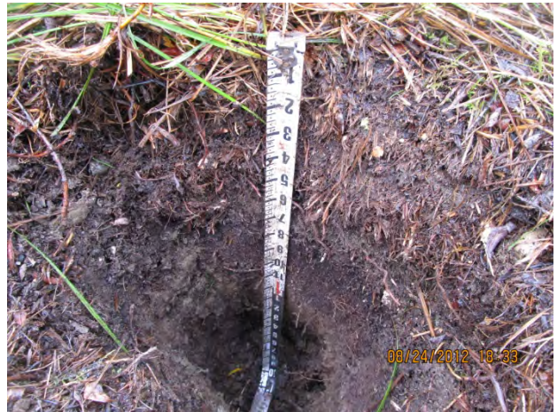
Hydrology: Saturation (A3) with a shallow aquitard (D3) Soils: Organics over silty clay loam (Histic Epipedon A2)
