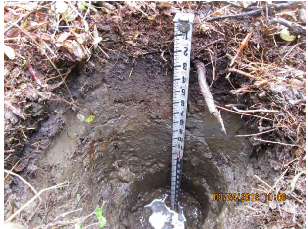
Hydrology: Saturated (A3) with high water table (A2) Soils: Organics over silty clay loam (Problematic, AK Gleyed)
