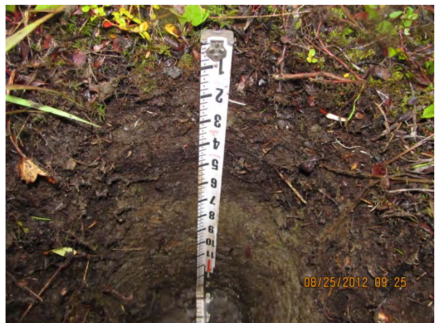
Hydrology: Shallow aquitard (D3) and FAC-neutral (D5) Soils: Organics over silty clay loam (Alaska Redox A14)
