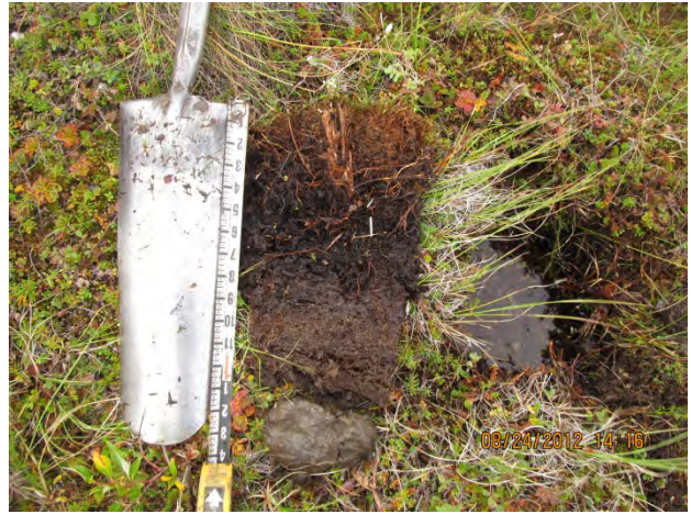
Hydrology: Saturation (A3) with high water table (A2) Soils: Organics over silty clay loam (Histic Epipedon A2)
