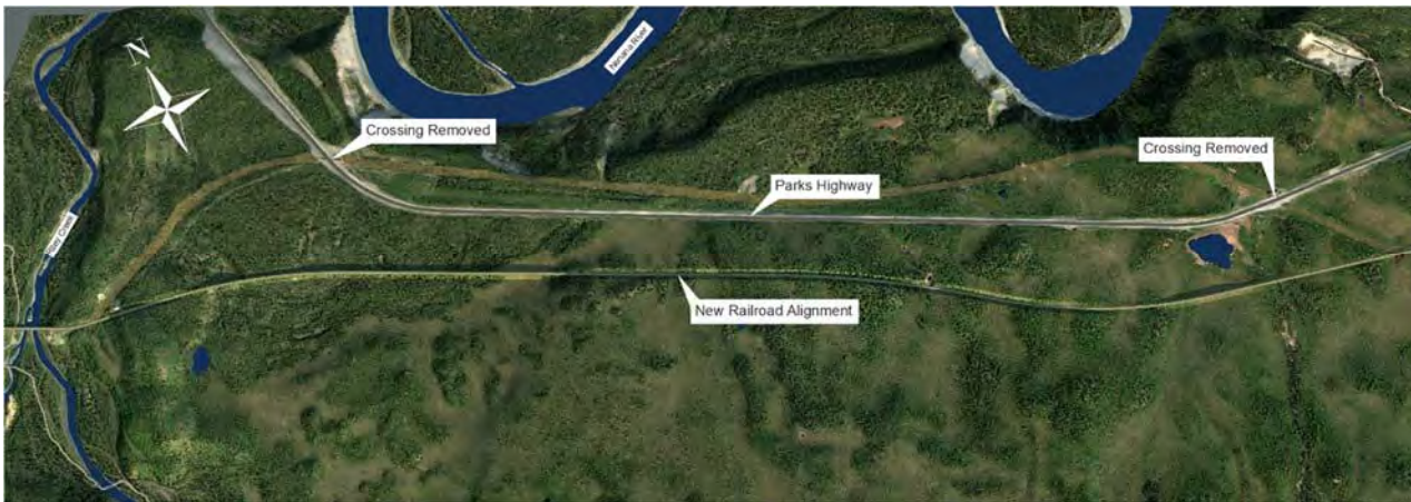
Railroad crossing solution #1 - potential realignment route
