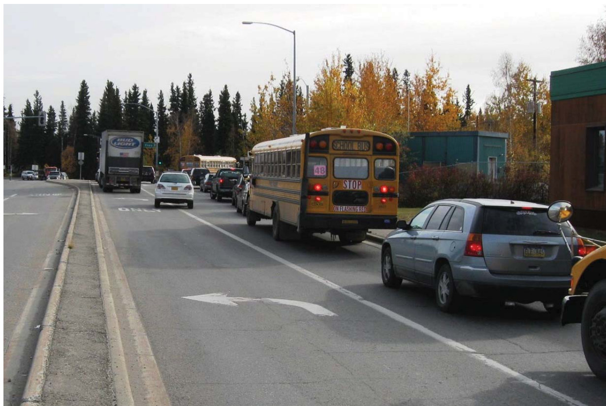
Figure 9. Eastbound Right Queues at College Road and Steese Expressway. Note the white car using the left turn lane to bypass the queued traffic.
