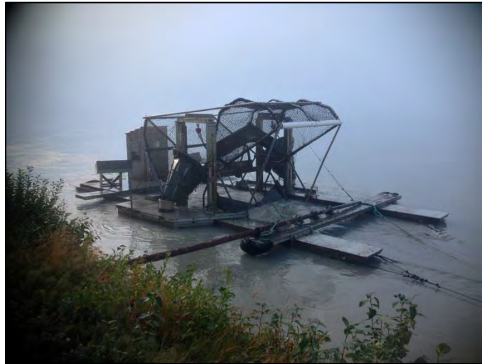
Figure 3. Typical fish wheel installation adjacent to Haines Highway. Note cable anchoring system and log pole used to position the fish wheel away from the bank.
