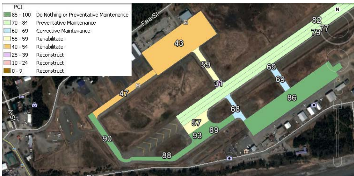
Exhibit 29. Airfield pavement condition
